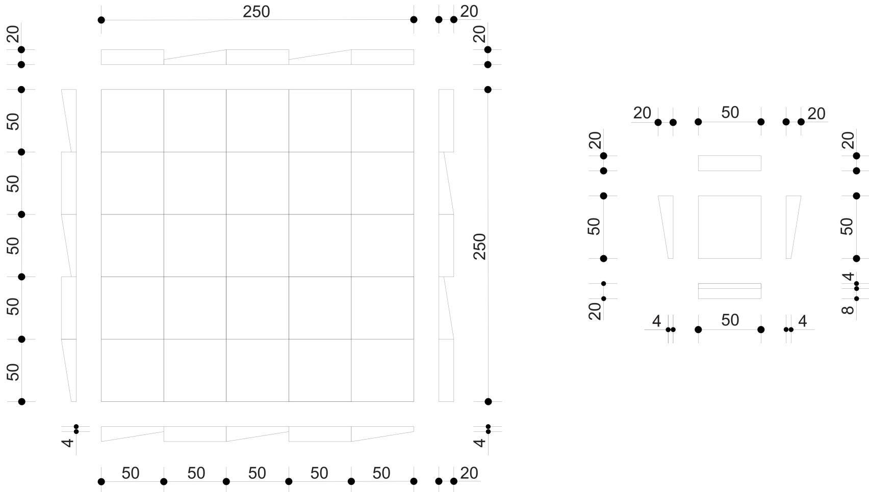
Massive cork piece, in 20mm, and 250x250mm exterior dimension.
